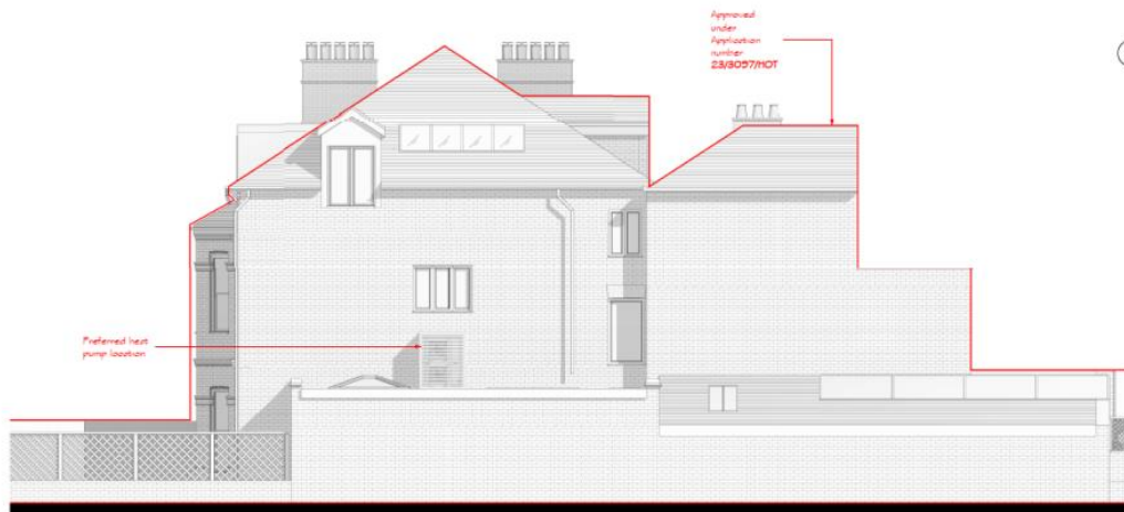
Figure 1 – Flank elevation showing proposed heat pump
