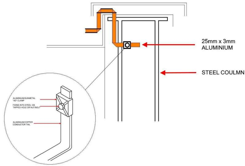
CONNECTION DETAIL TO STRUCTURAL STEEL
