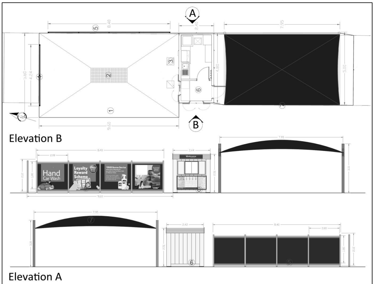
Figure 1 - Standard layout for a Waves car wash
