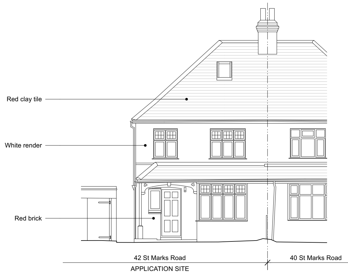
1 Existing Front Elevation Scale: 1:100
