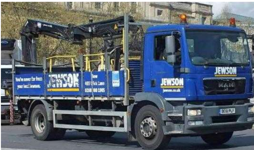
Standard Delivery Truck 7.5m (L) 2.6m (W) 2.8m (H)
