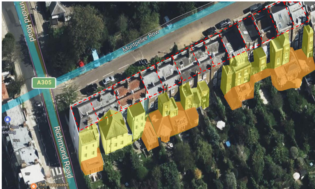
Figure 25 – Rear elevation of the entire terrace; Victorian (some with Georgian origins) closet-wings shown yellow. Modern extensions shown orange.
