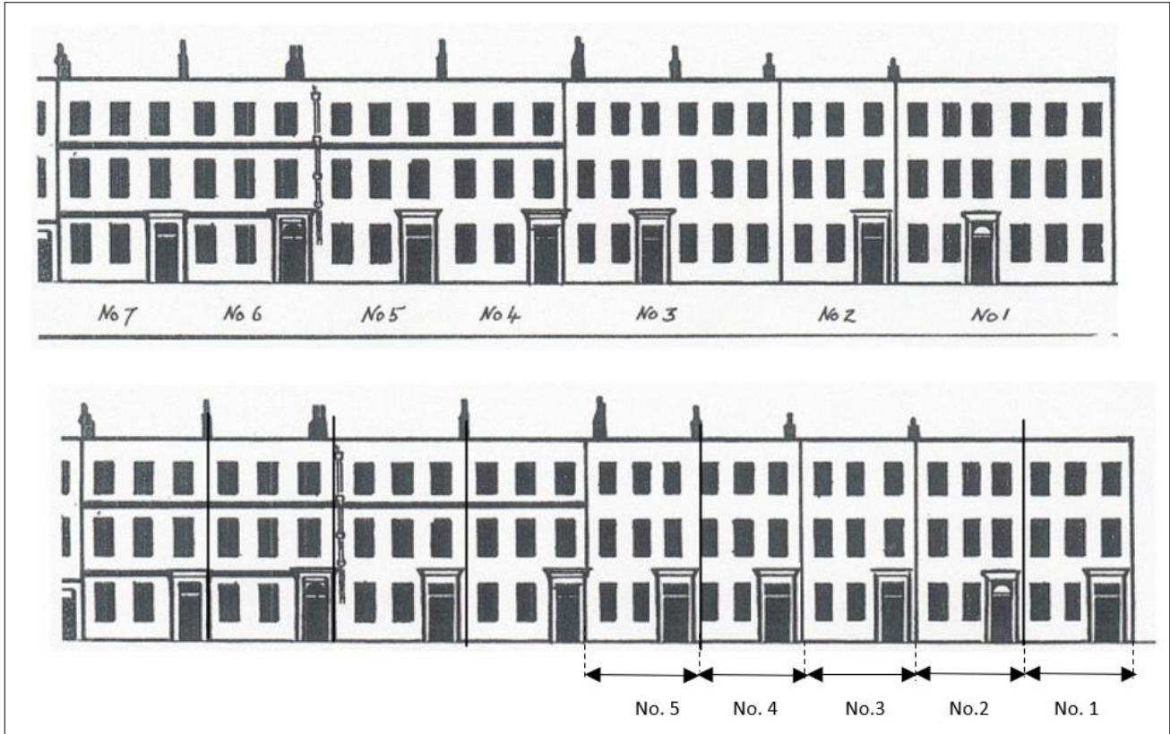
Figure 19 – Sketch layouts of Montpelier Row, W. Folds Hall, 1961: Original layout below; adjusted layout above
