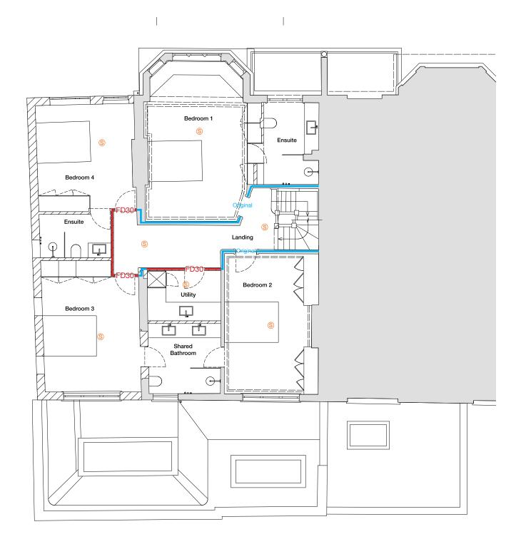
1:100 printed at A4. First floor plan.
