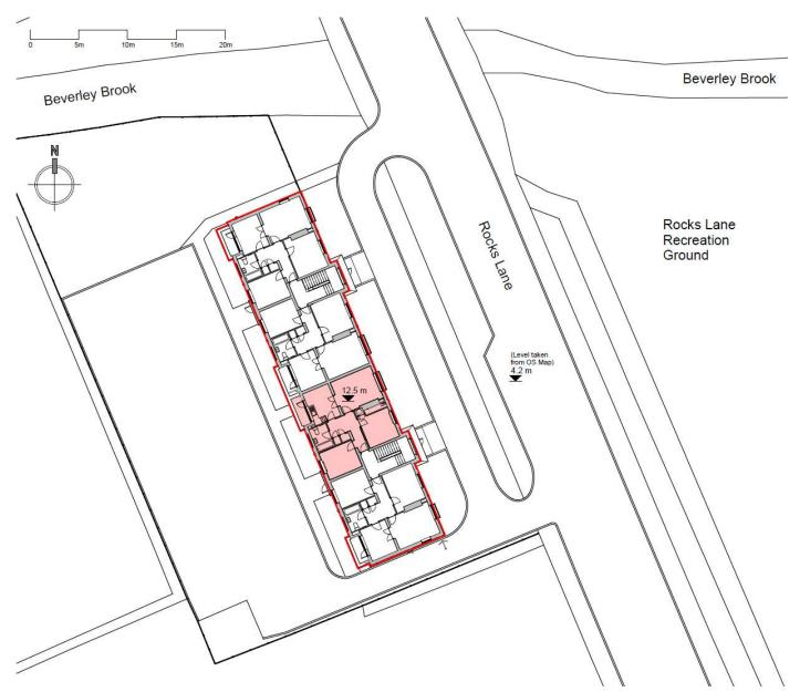
As is shown in the plan above the existing external ground level is 4.2m (taken from the Ordnance Survey Plan), while the finished floor level of the third floor apartment where the relocated boiler flue is being proposed is 12.5m, circa 8..3m difference.
