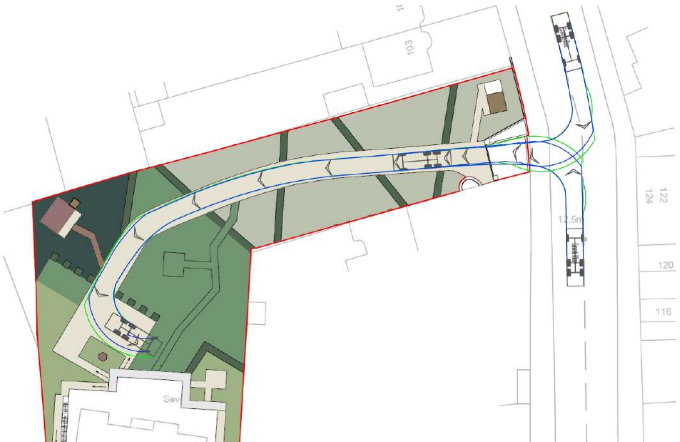
Figure 5 Construction Vehicle Swept Path Analysis – Concrete Mixer
