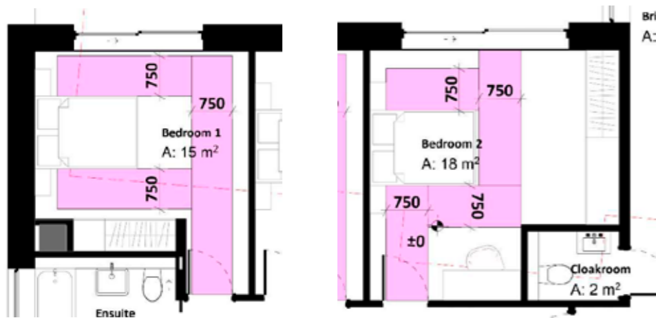
Above: Bedrooms 1 & 2 on the entrance storey demonstrating clear access routes of 750mm from the door to the window and all sides of the bed
