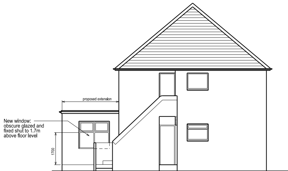
SIDE ELEVATION facing Nos. 78 & 80
