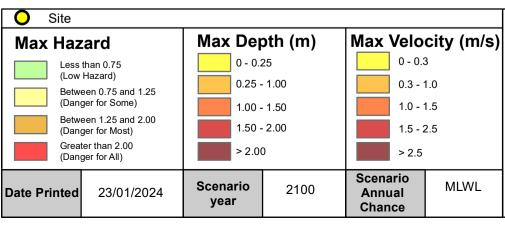
This map shows the combined flood hazard to people (called a hazard rating) if our flood defences are breached at any given single location, for a range of scenarios. The hazard rating depends on the depth and velocity of floodwater, and maximum values of these are also mapped.
