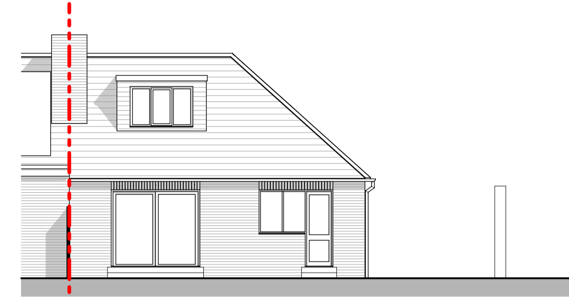
Existing Rear Elevation [North] Scale: 1:100
