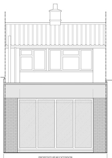
PROPOSED REAR EXTENSION — Brick to match existing with rendered parapet – Aluminium sliding windows
