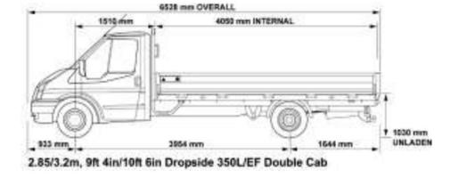
2.85/3.2m, 9R 4in/10R 6in Dropside 350L/EF Double Cab
