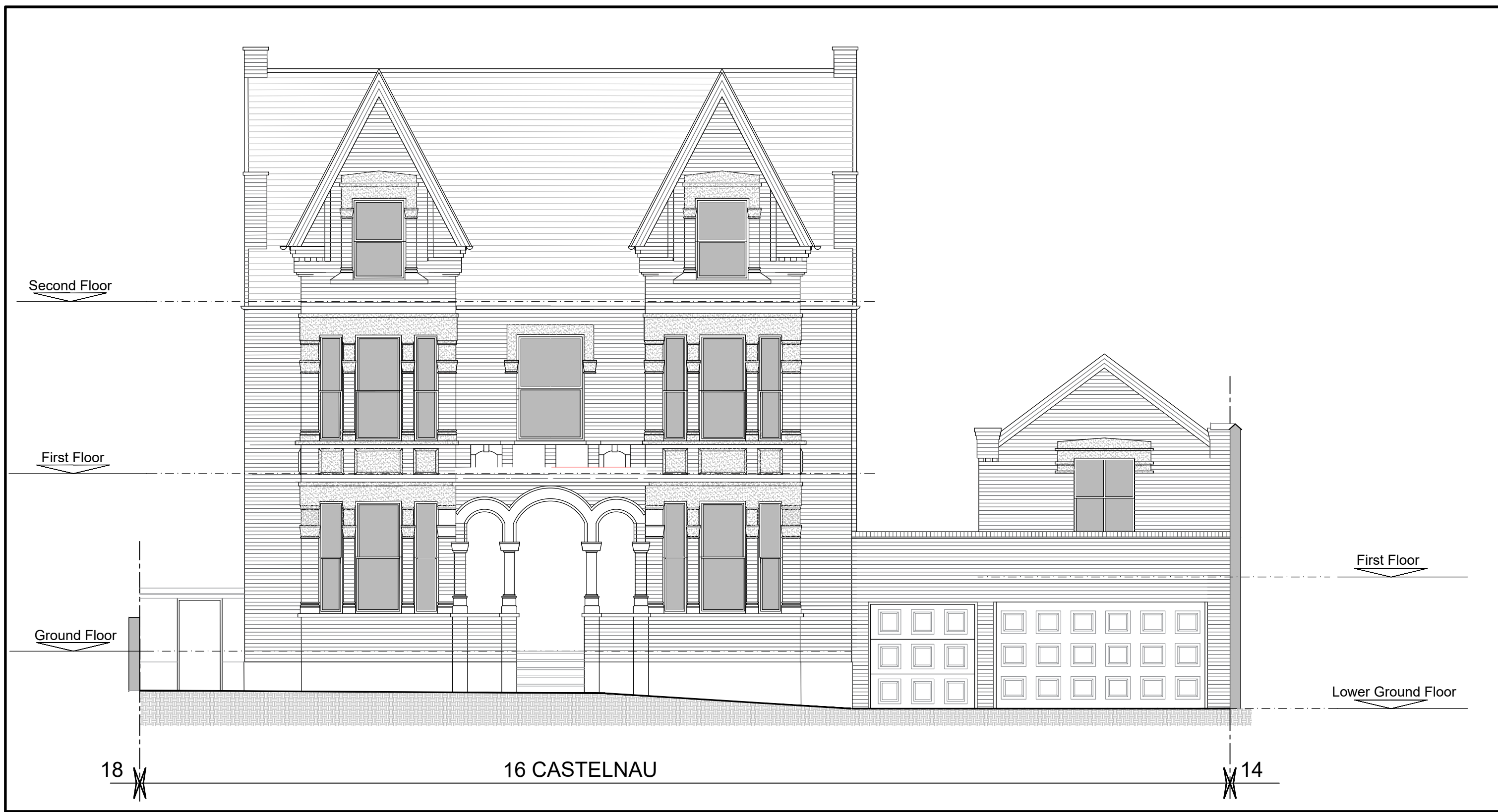
FRONT ELEVATION as EXISTING. Scale 1 to 75.
