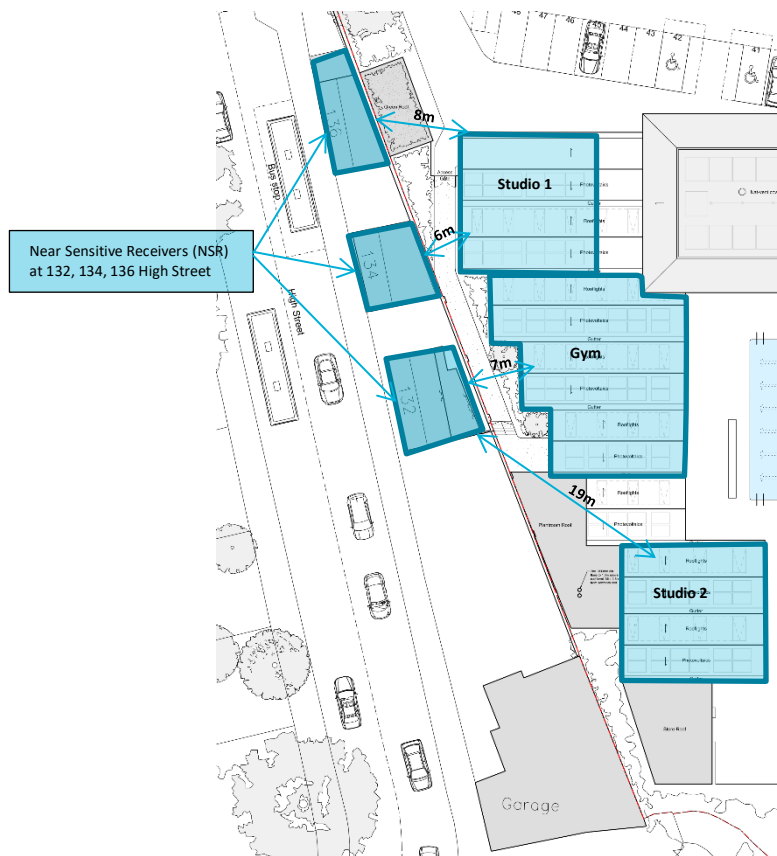
Figure 1 - Site layout showing the location of Hampton Pool Gym and Studios and nearest Sensitive Receivers (NSRs), 132, 134 and 136 High Street.
