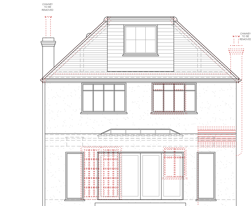
PROPOSED REAR ELEVATION Walls to be white render finish Roof to be in grey tiles Dormer wall - K Render finish
