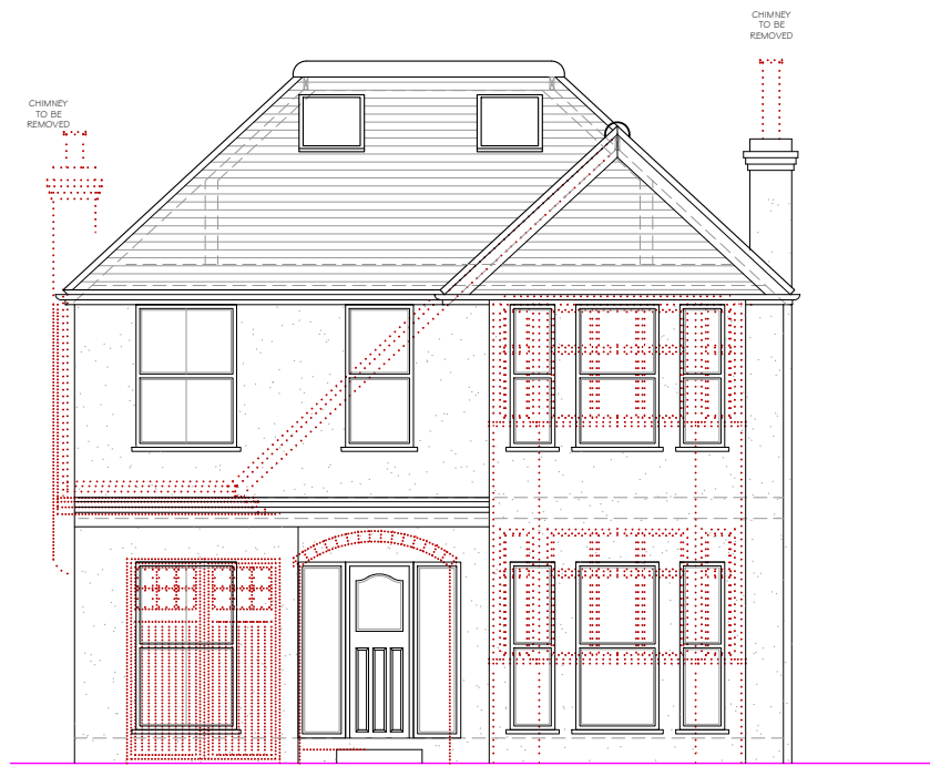
PROPOSED FRONT ELEVATION Walls to be white render finish Roof to be in grey tiles Dormer wall - K Render finish
