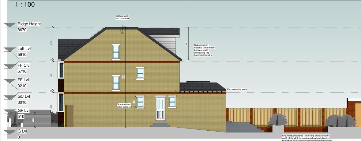
Ground level lowered (4.6m long and across the width of the plot) to match existing level directly behind house to comply and exceed compensatory flood risk requirements per the FRA
