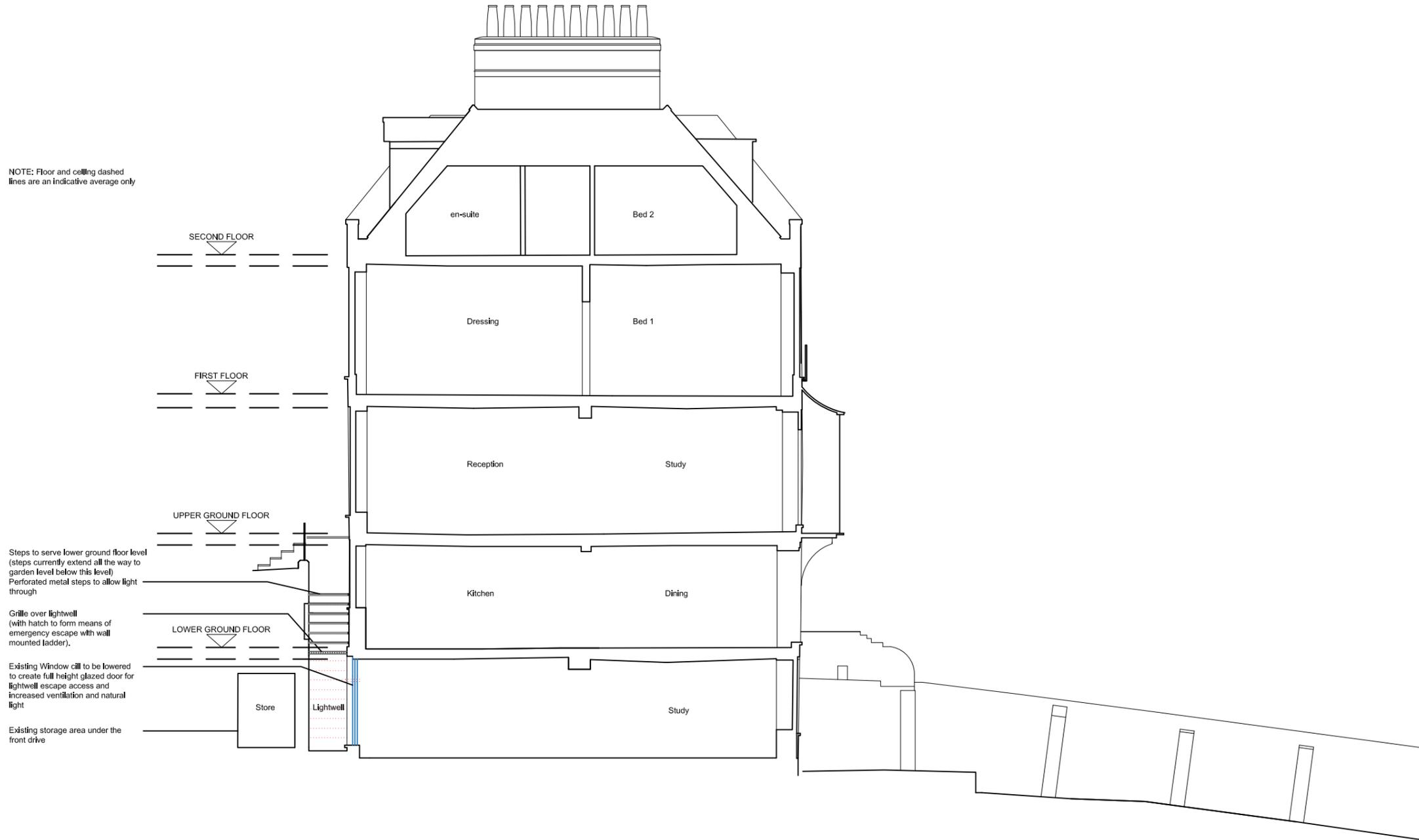
Steps to serve lower ground floor level (steps currently extend all the way to garden level below this level). Perforated metal steps to allow light through
