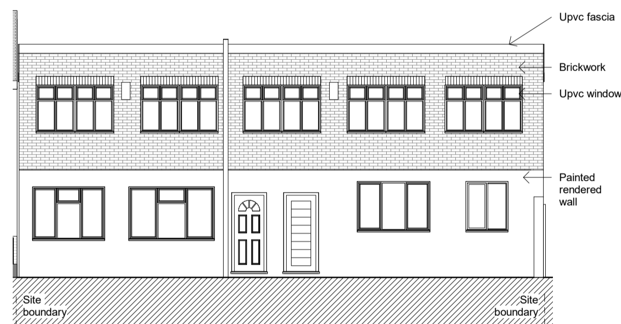
4 EXISTING FRONT ELEVATION (EAST) P301 1:100
