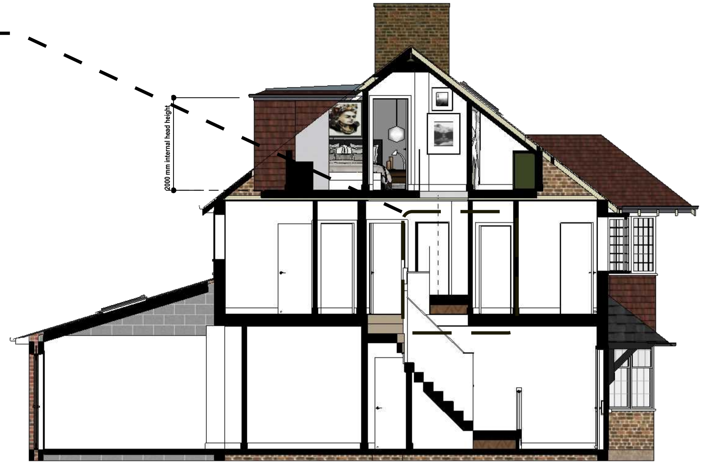
A 01 | PROPOSED SECTION B-B | scale: 1:50
