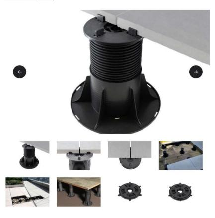
Paving Support | Fixed Head Adjustable Pedestal have 4mm spacer tabs to create a small gap between the Porcelain Paving slabs for drainage. These pedestals allow Porcelain Paving slabs to be set directly upon the head.
