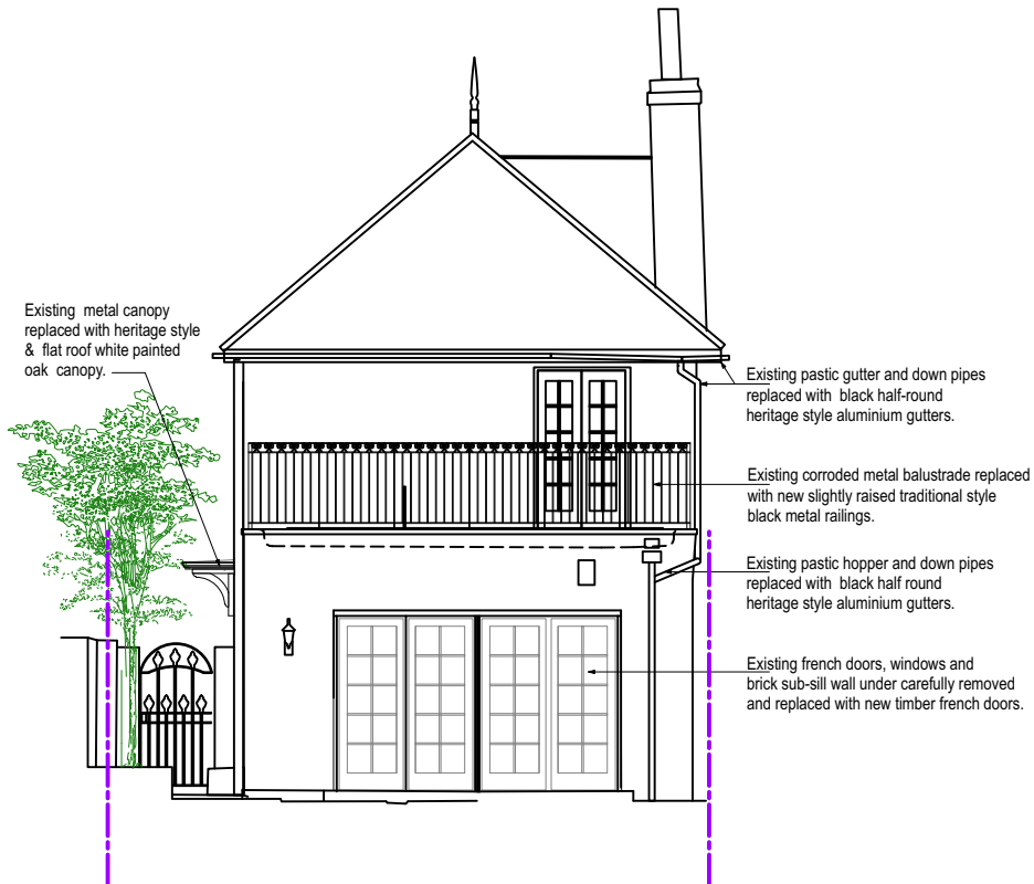
2 REAR ELEVATION MAIN BUILDING AS PROPOSED 1:100
