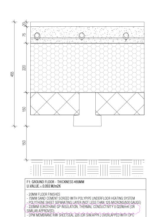
RETURNED UP THE BLOCK UPSTAND BELOW EXTERNAL WALLS AND GLUED TO WALL
