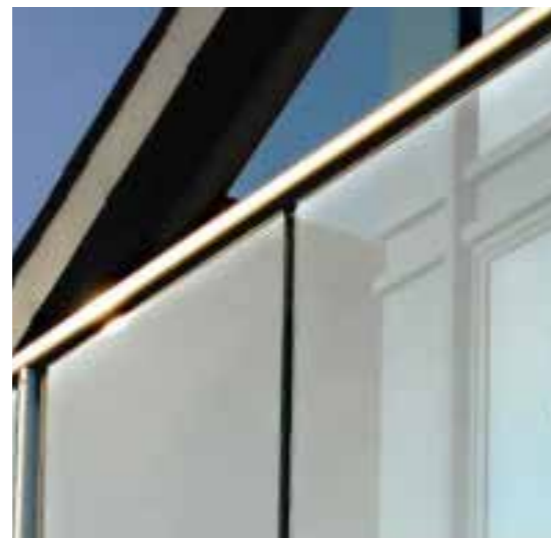
5. Glass Balustrades Glass balustrade in surface-mounted channel with clear 21.5mm laminated & toughened glass and brushed stainless steel handrail
