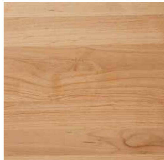
1. Glulam Structure visual finish Visual Grade Glulam (Douglas Fir or Spruce - dependant on supplier) treated with a water-based medium solid gel stain with very high UV protection to preserve the material's original appearance.
