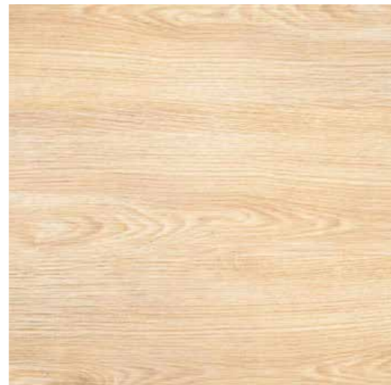
2. Visual plywood soffit Visual Grade plywood (Douglas Fir or Douglas Fir or Spruce - dependant on supplier) treated with a water-based medium solid gel stain with very high UV protection to preserve the material's original appearance.
