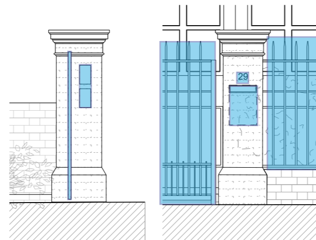
Proposed elevation - brick pier
