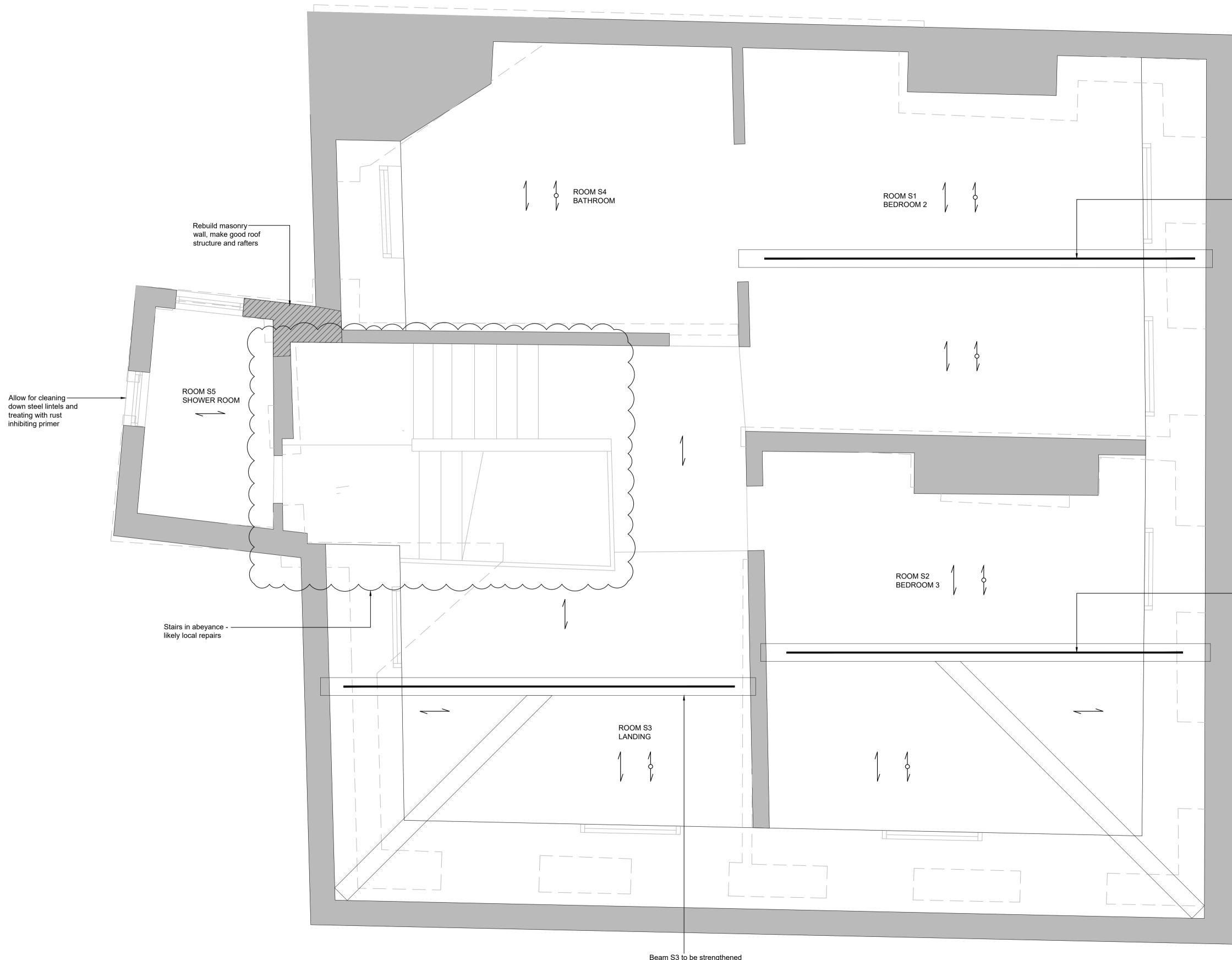
Beam S3 to be strengthened with steel flitch plate (size TBC). See typical detail on drawing (224260-MNP-XX-XX-DR-S-2105). General
