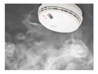
In line with Building control requirements, an interlinked smoke detection system will be installed to the outbuilding. This will mean smoke alarms on every level, interlinked so that when one sounds they all sound. This will also be linked to a heat detector in the kitchen.
