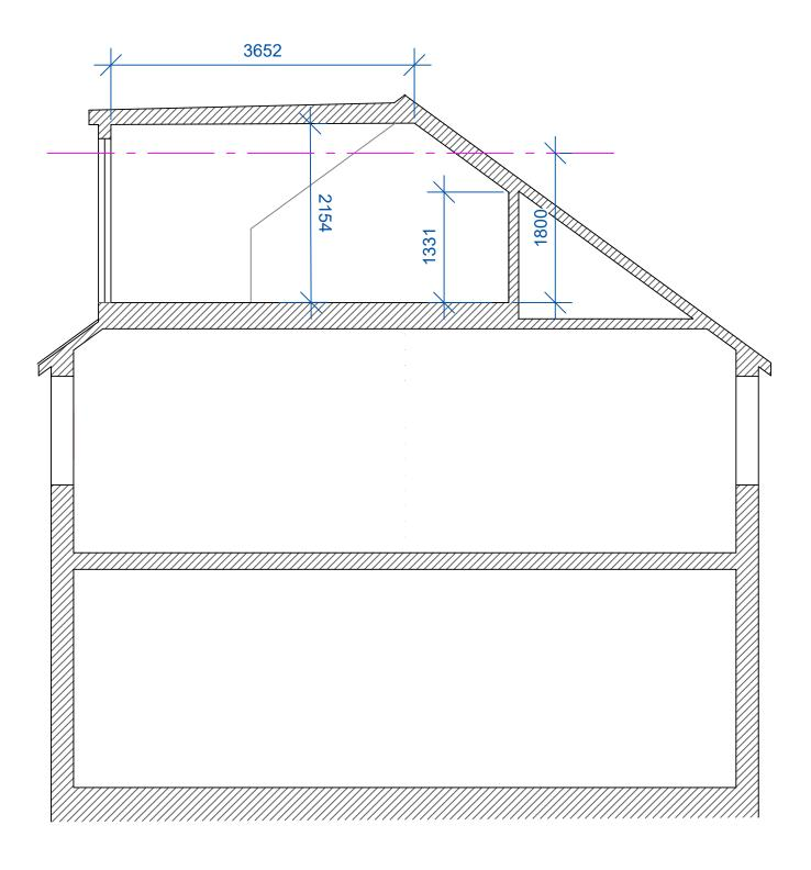
Typical Section through Proposed Loft Conversion
