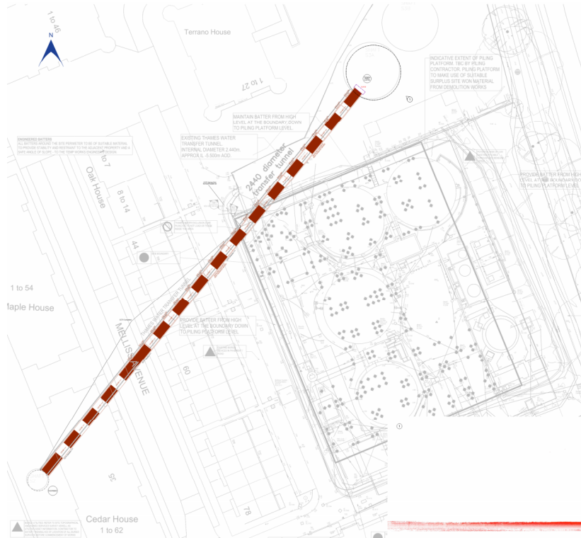
Figure 2-1 – Surveyed position of the tunnel
