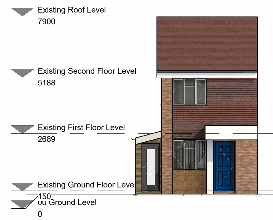
Existing Front Elevation 1 : 100
