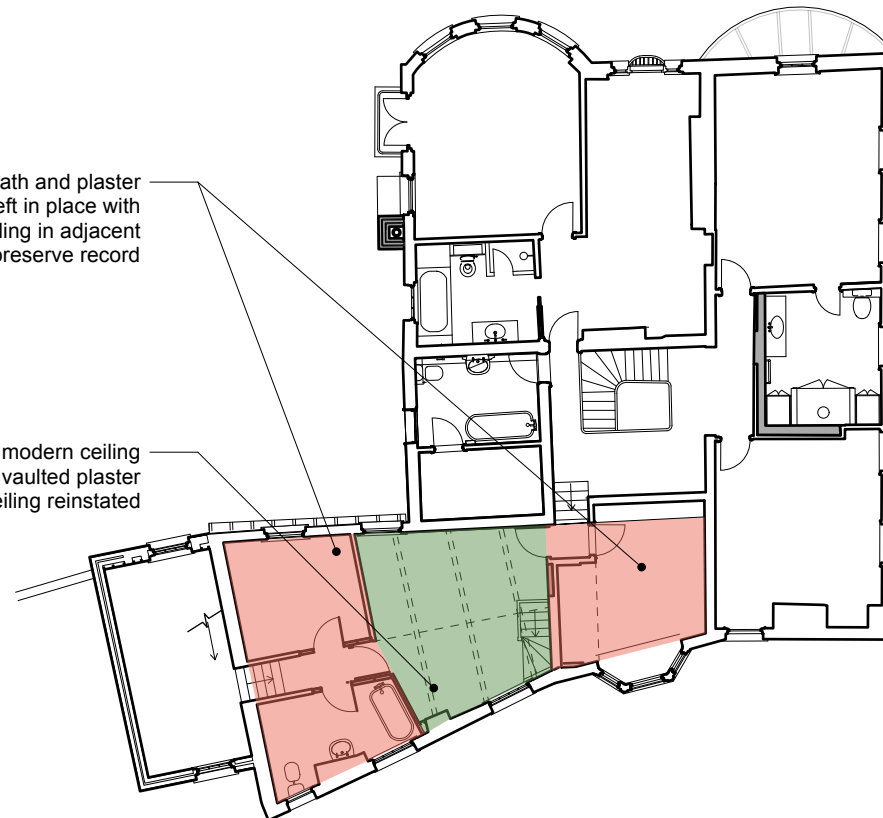
Proposed First Floor Plan - Scale 1:200 Showing extents of existing and proposed vaulted ceilings
