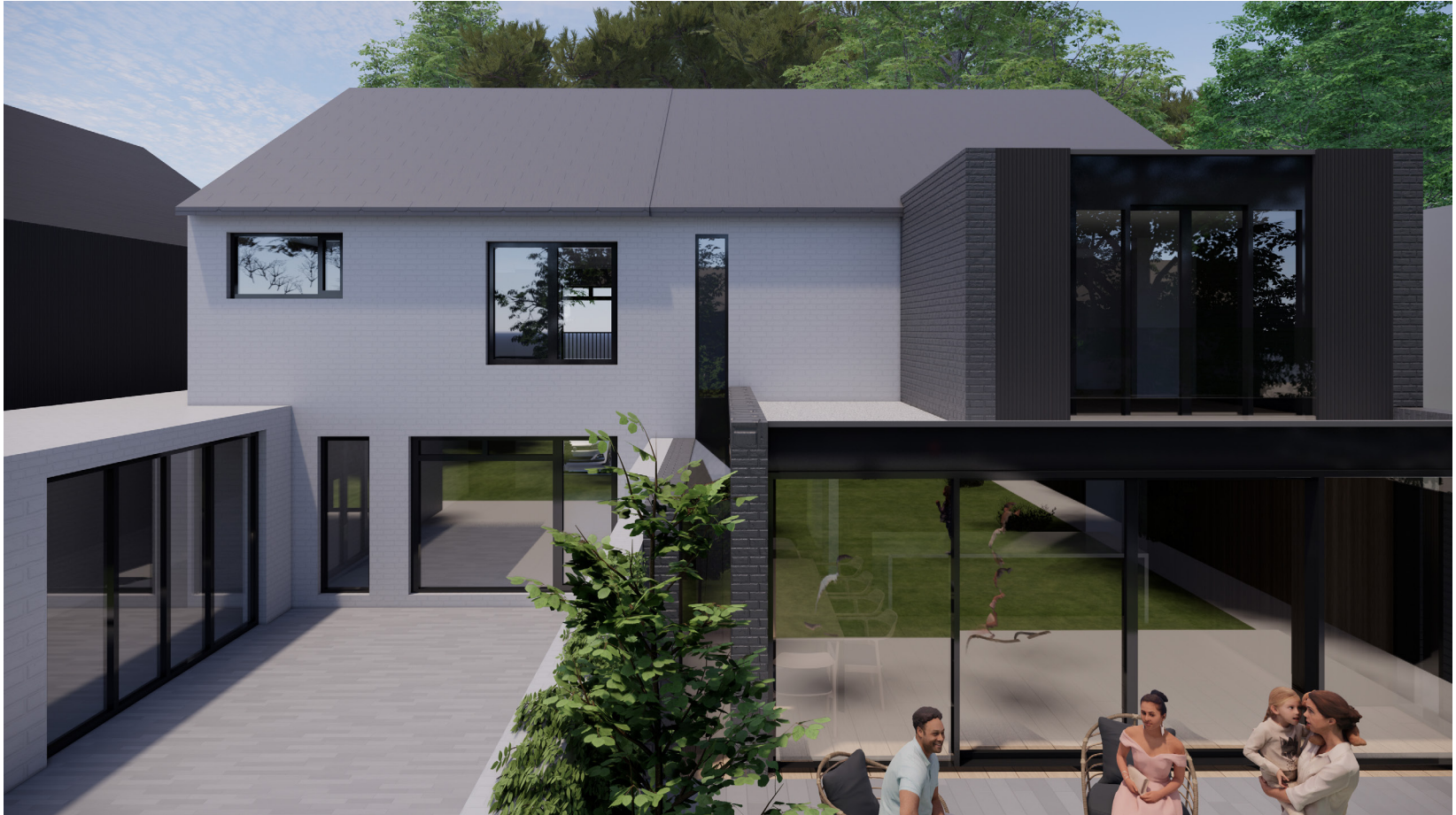
The set back design articulation around the existing boundary wall enables the proposed rear extension for 94 Temple Sheen to comply with the 25 degree rule.
