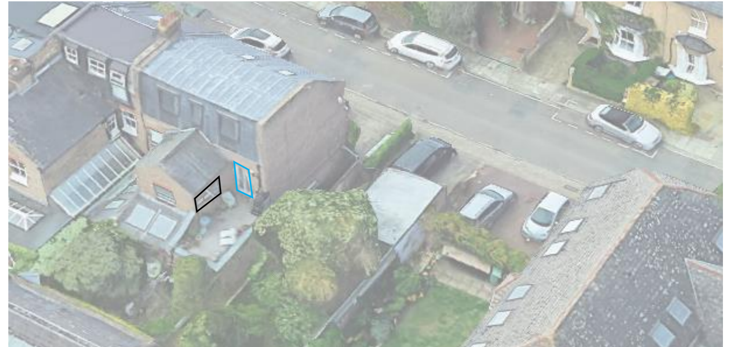
Figure 7. Main windows assessed on 5 Ellison Road (source: Google Maps). Windows marked in black were modelled in detail while the window marked in blue was found to pass BRE's initial tests.
