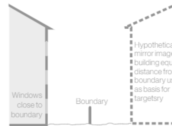
Figure 12: Mirror image methodology (source BRE guide 2022)
