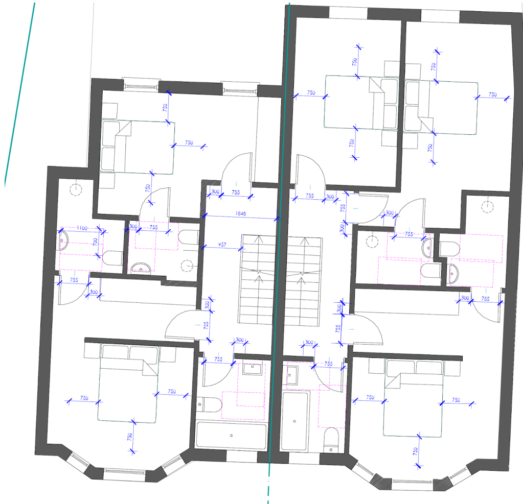
Fig. 8: Plots 1 and 2 proposed first floor circulation space, min 1848 mm wide. Proposed plans of all bedrooms with dimensions showing minimum clear space around the bed. Extract from drawing 2041.03.03.Pln01.023.
