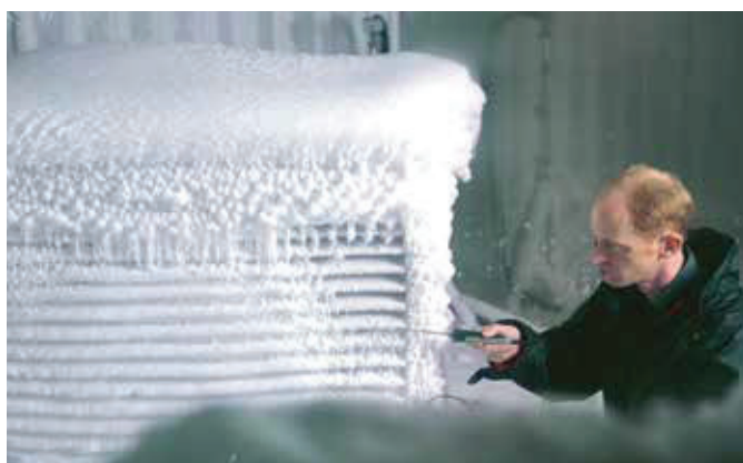
Climatic chambers simulate all possible operating conditions
