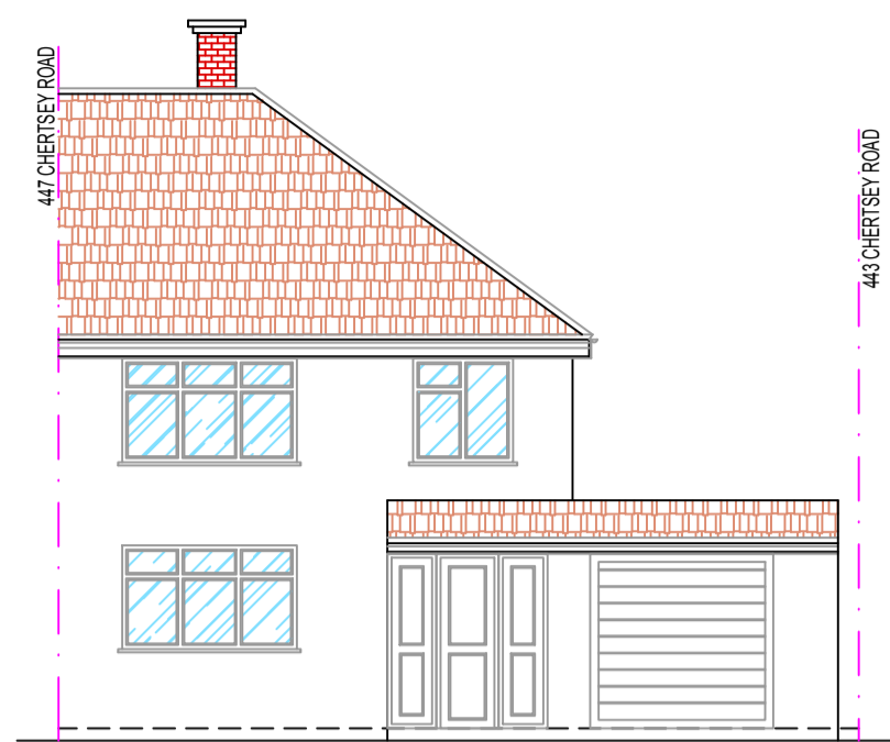
EXISTING FRONT ELEVATION SCALE 1:100@A1
