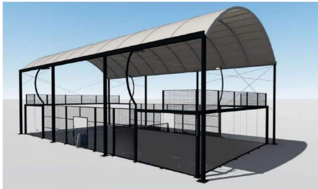
Figure 3: 3D Image showing Typical Padel Court Canopy
