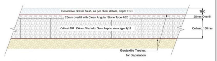
Note: Subbase could be required depending on the existing ground CBR % and the type of traffic on the surface.
