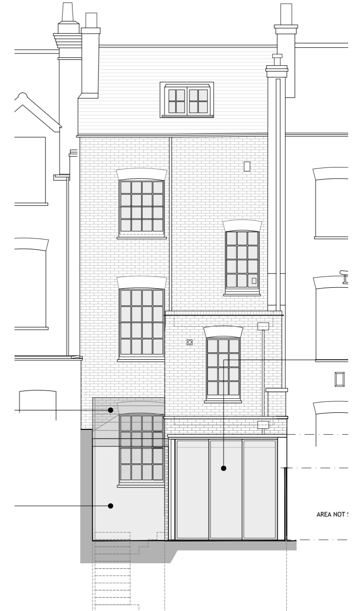
Proposed Scheme | Rear Elevation - Visually maintains relationship of solid/void when viewed from within rear garden. Low level brick wall and returning stairs removed
