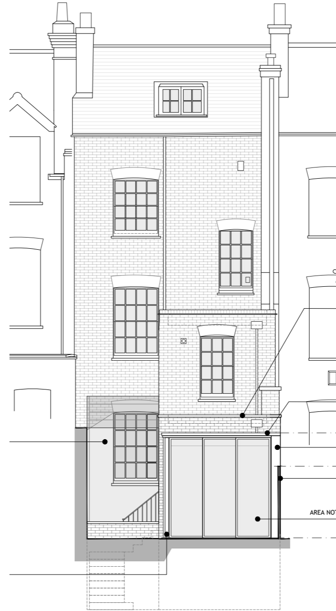
Approved Scheme Combined | Rear Elevation - Half width rear extension, side infill with low level brick wall. Internal stair returning into kitchen
