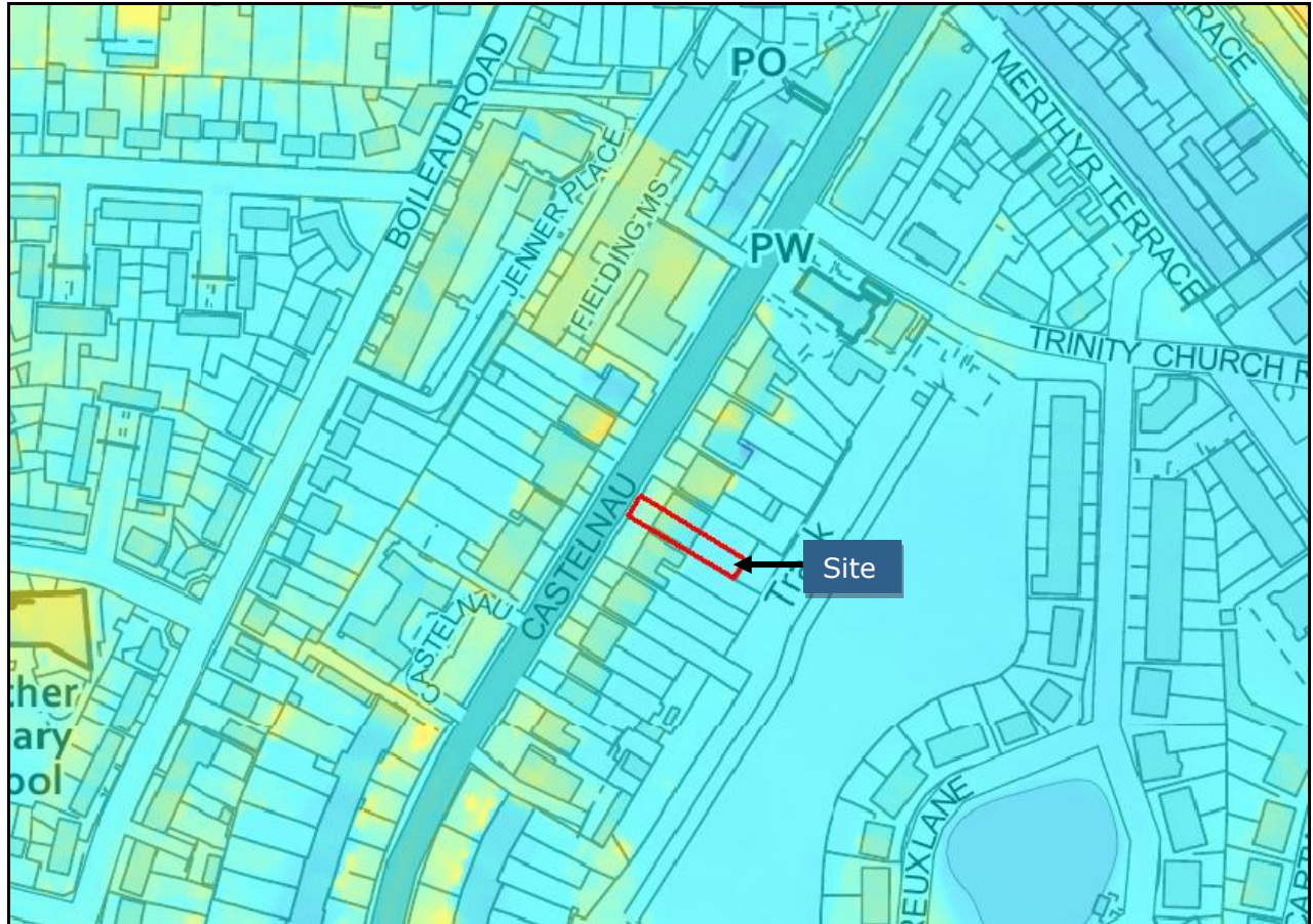
Figure 2: Filtered 1m LIDAR survey data where higher ground is denoted as orange and yellow colours and lower areas denoted by blue and green colours
