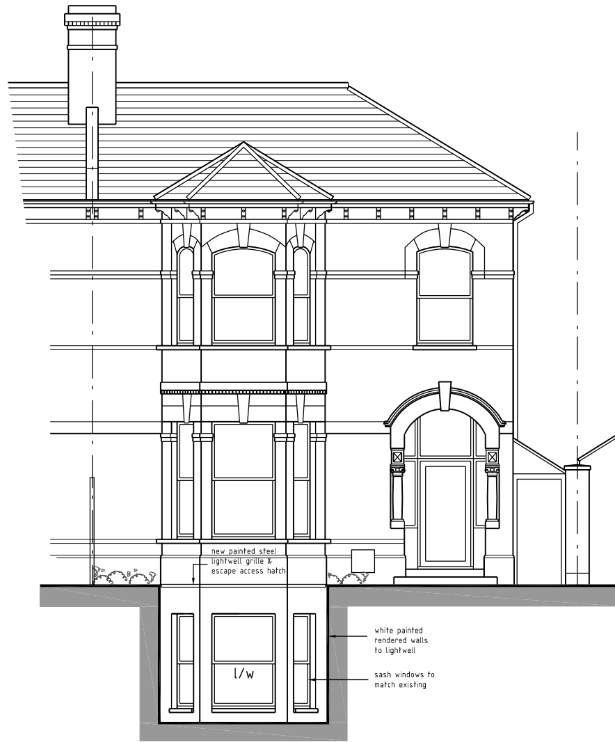
FRONT ELEVATION (sectional)
