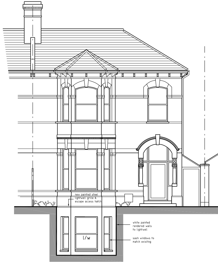
FRONT ELEVATION (sectional)
