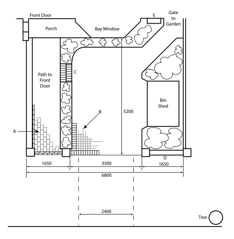
A = Pathway constucted out of pourus block paving
