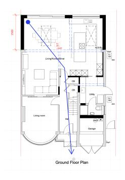
Figure 1.0 - route totalling 14.5m. Dedicated Evacuation Route, Floor Plans – Blue line denotes proposed escape
