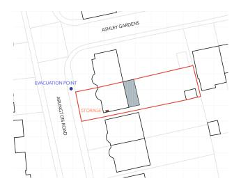
Figure 1.1 - Site Plan Demonstrating Evacuation Zone and Unobstructed Area for the Storage of Fire Equipment
