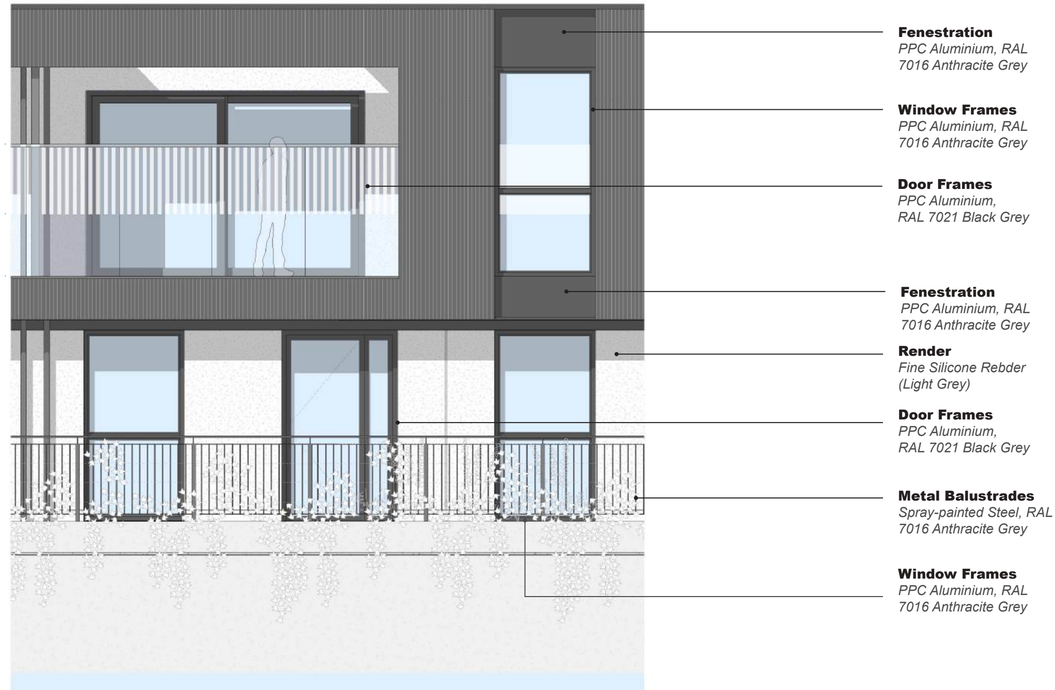
Detail Elavation - Rear Building East Scale 1:50 @ A3
