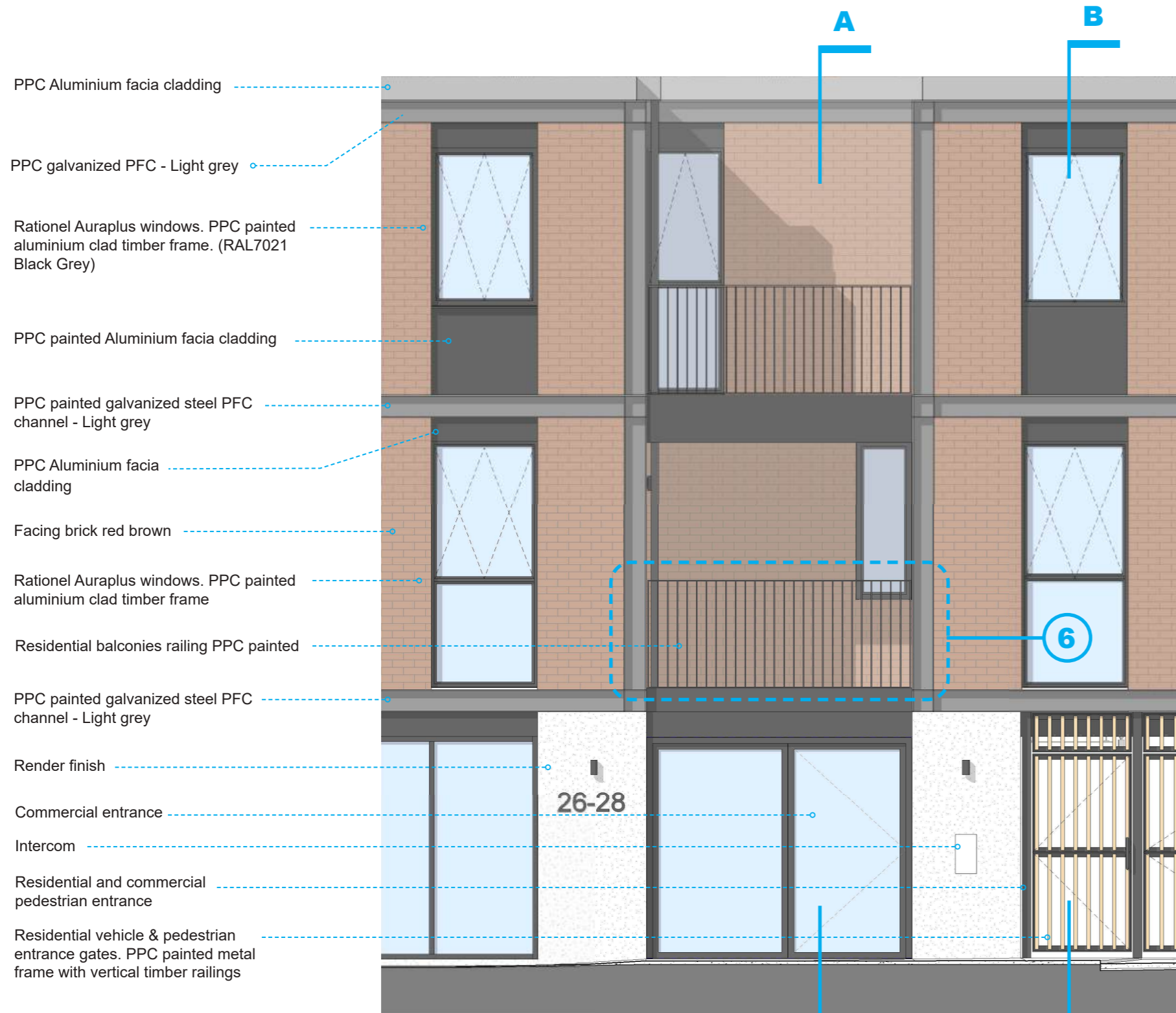
Detail Elevation - Front Building South Scale 1:50 @ A3
