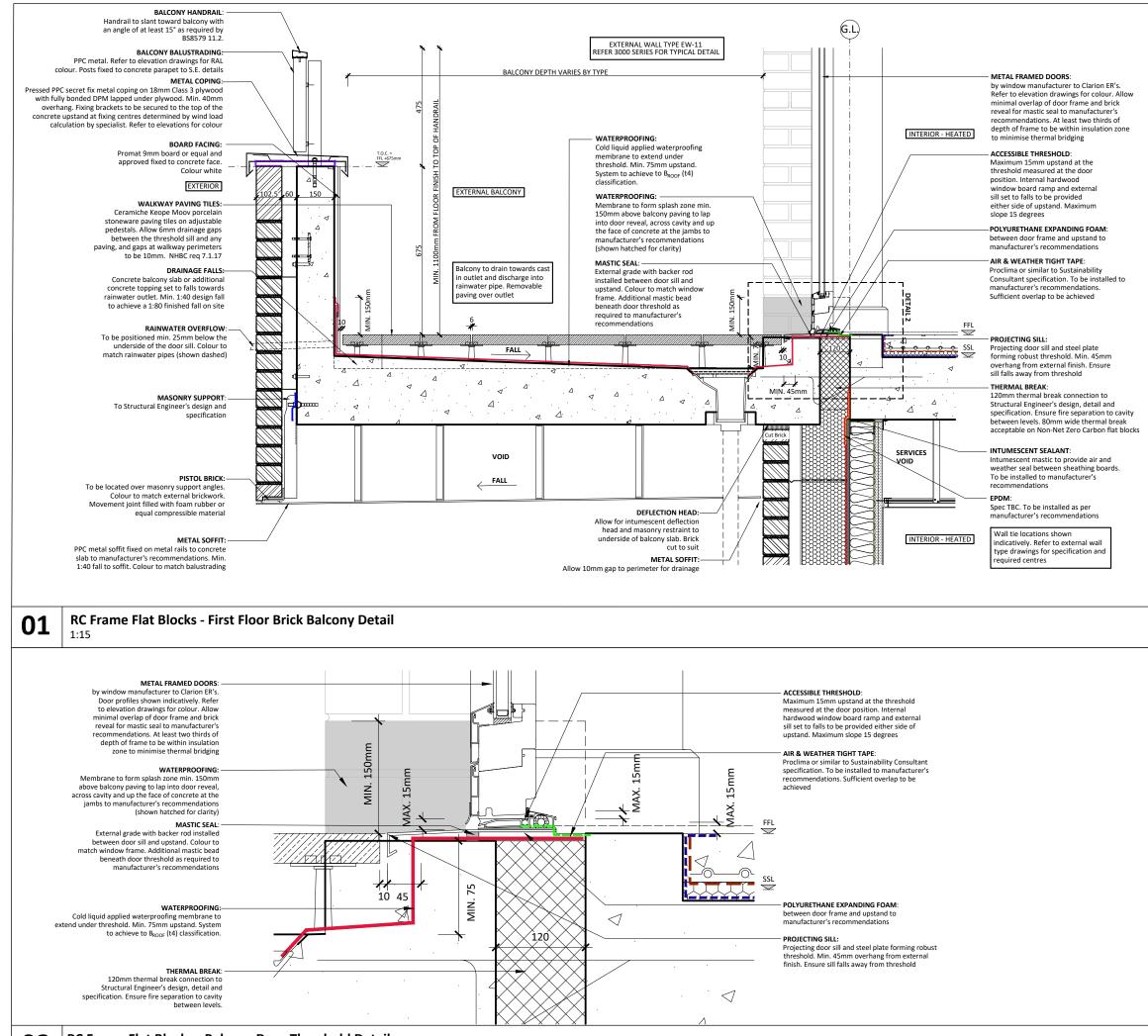
**RC Frame Flat Blocks - Balcony Door Threshold Detail**
