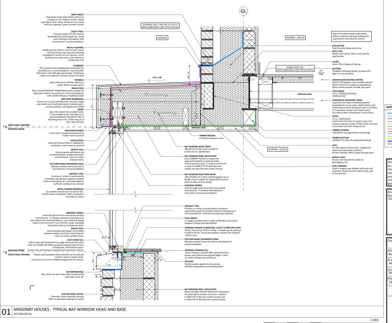
MEMBRANES KEY DPC to cavity/fire barriers Waterproofing Layer Tanking Primer Detailing Cover Strip Air and Vapour Control Layer (AVCL) ---- Breather Membrane Seperating membrane EPDM Airtightness Tape Flexible Foil Seal Fixing Strip Acoustic Resilient Layer
