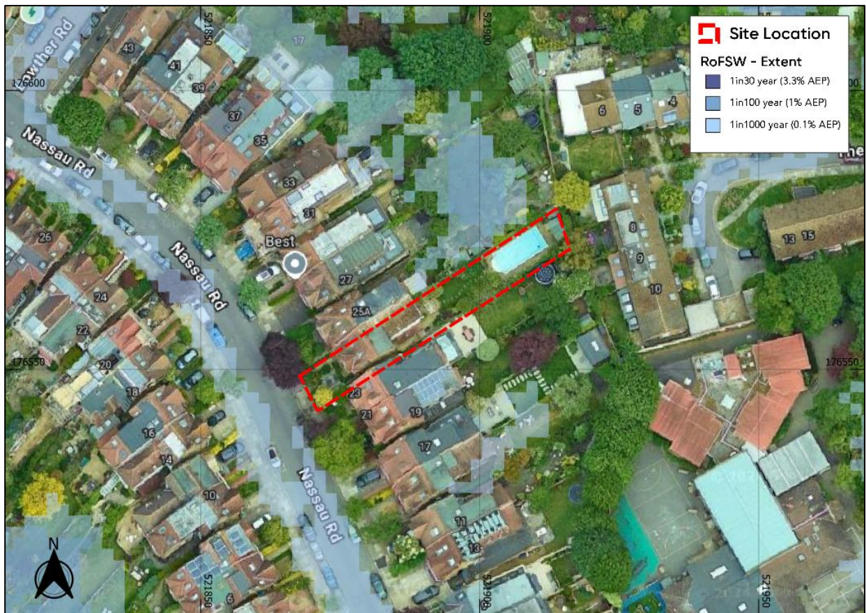
Figure 7: EA Surface Water Flood Risk Mapping (Base map and data from Google Satellite Imagery. Contains public sector information licensed under the Open Government Licence v3.0)
